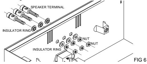
**HINT** : For easy fastening of the speaker terminals, immobilise the terminal by inserting a screwdriver in the wire hole, while fastening the nuts.
