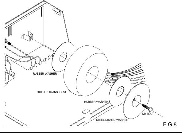
IMPORTANT: Do not trim the wires of the transformers, leave them at their original length. If there is more than one conductor in an insulating sleeve, you have to make sure they are soldered together and make a good electrical connection before they are connected to the terminal block.
