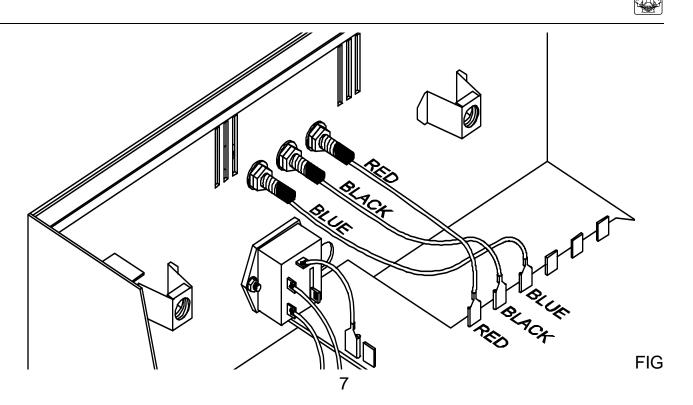
• Mounting of the toroid transformers : The output transformer marked ZD043 must be fitted according to the illustration, on the right hand side of the cabinet. Watch the location of the wires.
