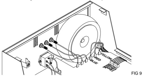
The supply transformer must be fitted according to the illustration, on the left hand side of the cabinet. Watch the location of the wires. The sturdy grey and green wires, which supply the 6,3V filament voltage, must sit on top.
