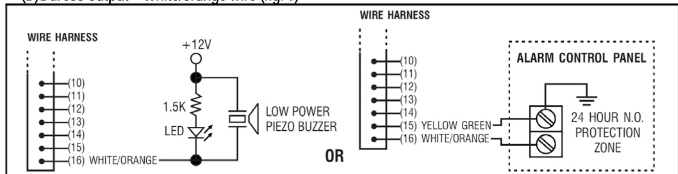
The duress output will switch to (-) ground when the duress code is entered. You may use it to turn on an LED lamp and/or a small buzzer. Connect it to a N.C. 24-hour protection zone of an alarm system.
