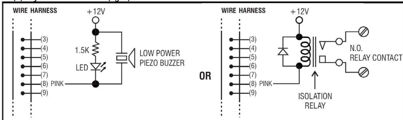
The key-active output will switch to (-) ground for 10 seconds whenever a key is pressed. Use it to turn on an LED lamp and/or a small buzzer to notify a guard, to energize a relay to switch on lights or a CCTV camera...
